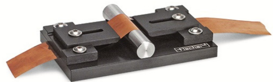
Fig. 2: Foil clamping device for securely holding thin plastic or metal foils
