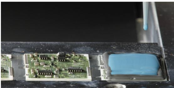
Fig. 1: "Glob top" application of a conformal coating on a PCB
