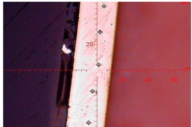
Fig.2: Indents performed precisely at the center of cross-sectioned layer
