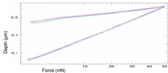
Fig.3: The graph shows reproducible load-displacement curves from each indent in Fig. 2.
