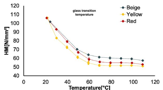
Fig. 2: Martens hardness of a thermoplastic in different colour variations as a function of temperature
